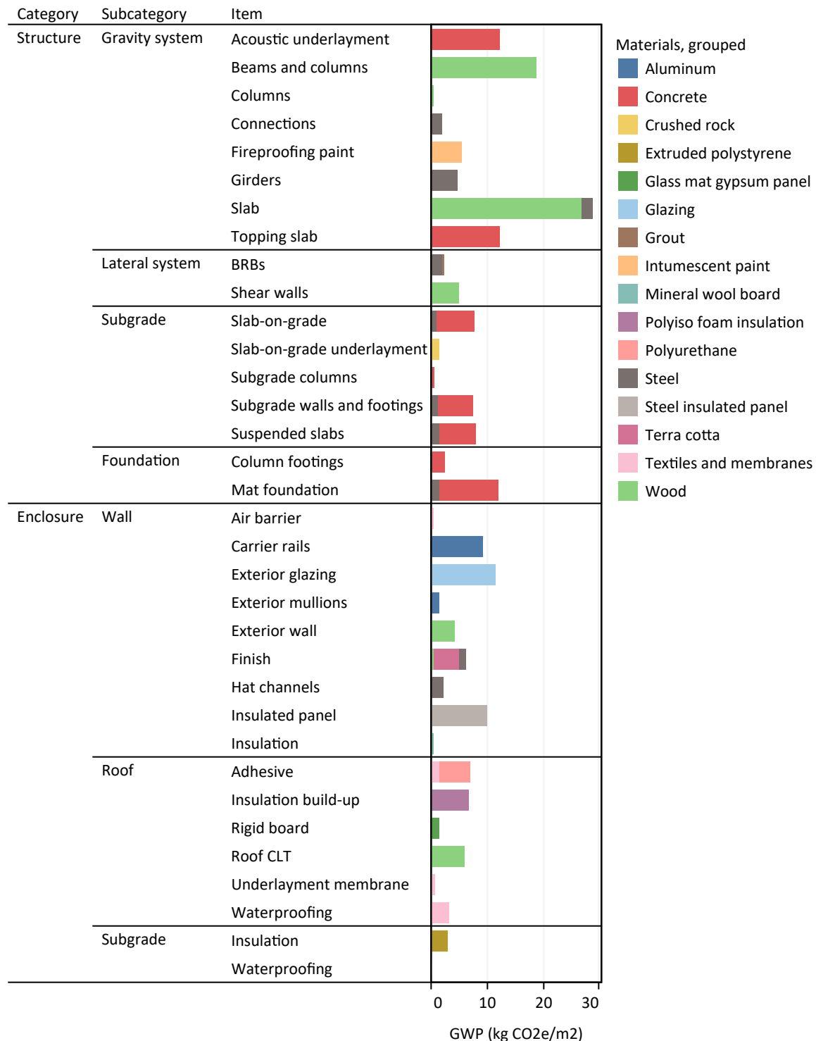
Figure 4. GWP results (life cycle stage A) of Catalyst Building LCA, normalized by total floor area of the building.
